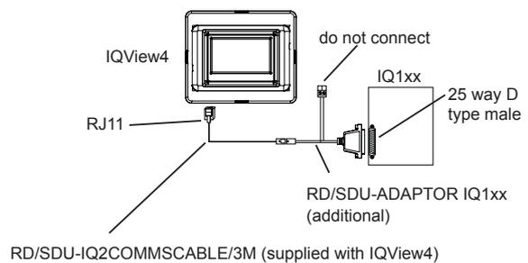
Some IQ1xx's have a 5 way in-line local supervisor port connector which can be connected using an additional adaptor cable (RD/SDU-ADAPTORIQ1xx+)
