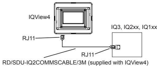
The signal connection to IQ1xx controllers with a 25 way socket requires an additional adaptor cable (RD/SDU-ADAPTORIQ1xx).
