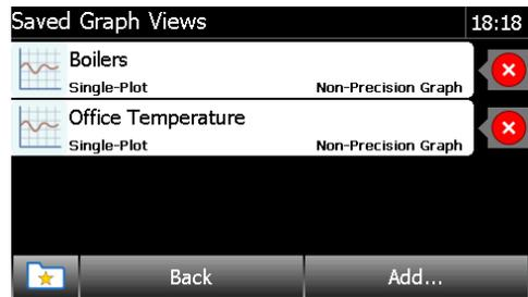
**Add...:** This enables the definition of a graph from a plot module in the controller to be added to the saved graphs. Selecting a saved graph shows the graph view.
