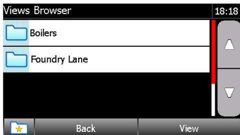
Selecting a directory module will display the modules pre-configured in the controller's display modules.
