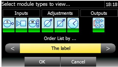
Module types can be selected or de-selected by clicking on the icons; a selected module type will have an icon with a green bar at the bottom.
