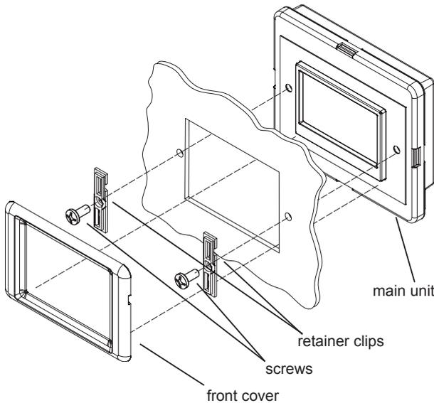
The display panel assembly consists of the main unit, 2 retainer clips and screws, and a front cover.
