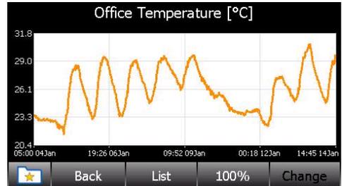
Dragging the finger over an area of graph will zoom to that area. : The left or right hand arrows enable the individual traces to be selected.
