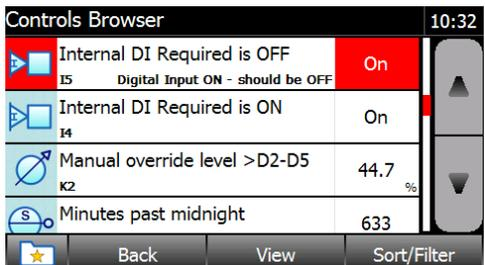
The large arrows on the right of the screen allow the user to scroll up and down the list.
