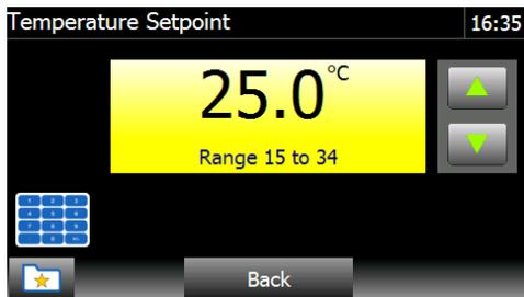
The above display is a knob module details page. It enables the knob value to be adjusted either by selecting the up or down arrow keys which allow increments/decrements of 0.1. As the value is changed on the screen, the value in the in the controller is updated.
