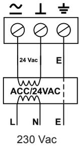
using 230V/24V ac transformer with one side earthed (grounded)
