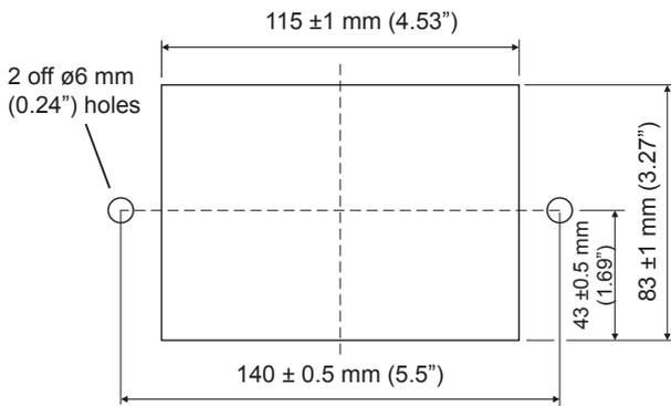
The panel should be pieced with a square cutout for the display, and drilled with two 6 mm (0.24") holes for the screws.
