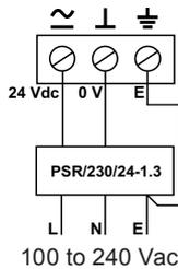
Some transformers are earthed on one side of the secondary. If so ensure the earthed side is connected to the central terminal of the power connector. If the polarity of the connection is incorrect the unit will not power up. If this happens swap left and central connectors
